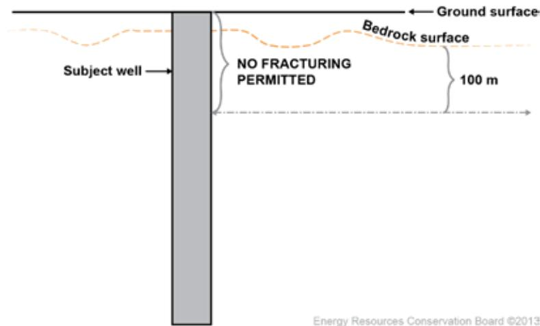
Figure 4. Hydraulic fracturing near top of bedrock.
