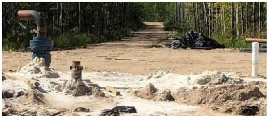
**Figure 3.** Sand extraction pump and PVC monitoring well at Vivian MB
